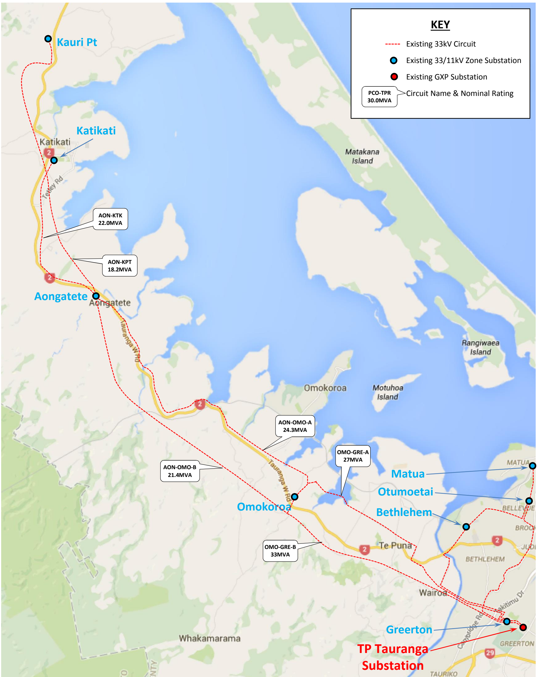
Figure 1 Existing Omokoroa/Aongatete/Katikati/Kauri Pt Sub-transmission Network: Geographic Diagram 7
