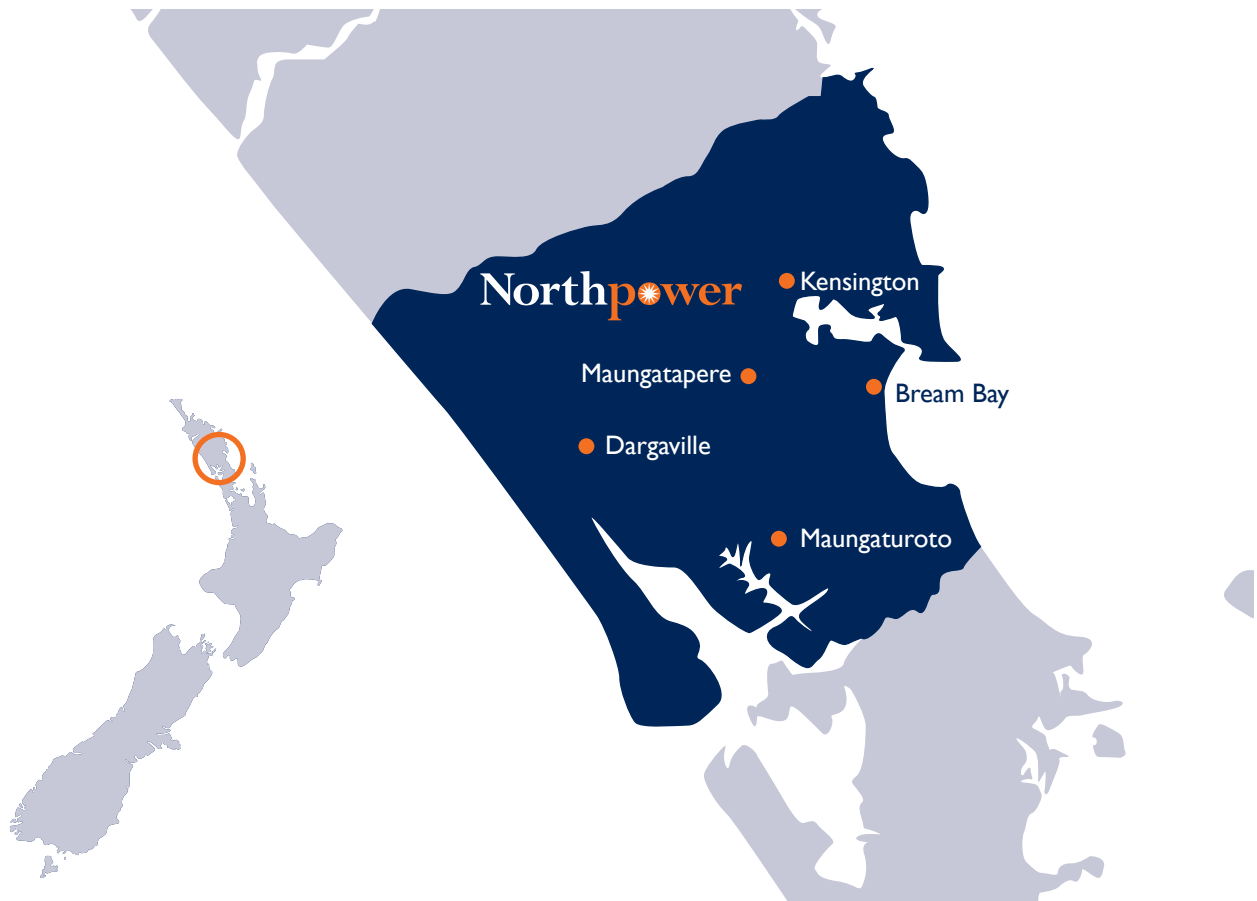
Northpower geographical area of supply and major substations
