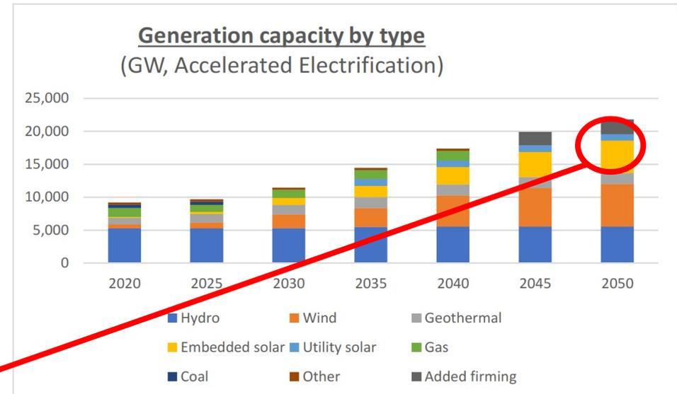
Transpower's 2050 future has 5GW of solar on around a third of residential properties (788,000 ICPs) between 4 and 5 kW each
