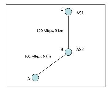
Note: The radial distances from A - B and B - C must be calculated separately and added together to determine the applicable distance group for the Links from A - C.
