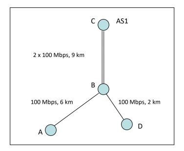
Note: The radial distances from A - B and B - C must be calculated separately and added together to determine the distance for the Links from A - C. Similarly, the radial distances from D - B and B - C must be calculated separately and added together to determine the applicable distance group for the Links from D - C.
