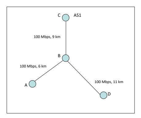
Note: the radial distances from A - B and B - C must be calculated separately and added together (as these are the links that were first purchased) to determine the applicable distance group for the Links from A - C. The radial distance from D-B is then used to determine the applicable distance group for the Link from D - B.
