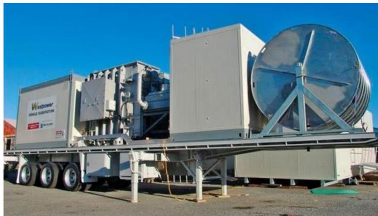
Figure 8 – Mobile Substation
