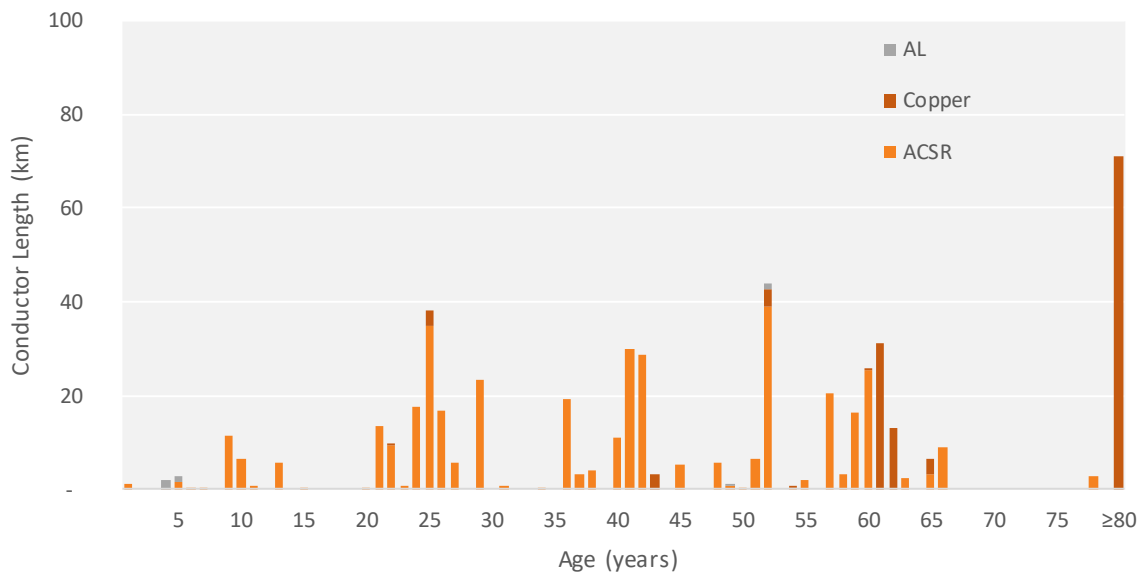
Figure 8.18: Subtransmission conductor age profile
