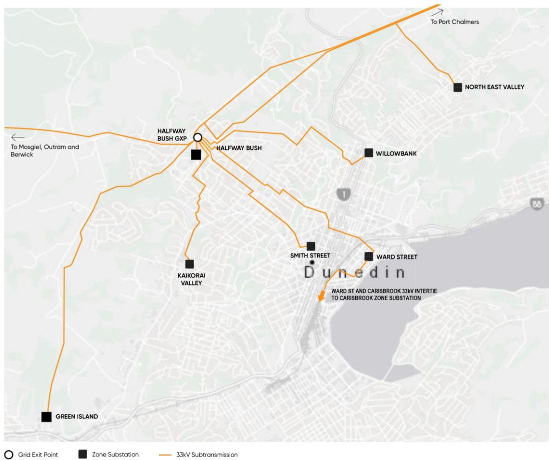
Figure 3.6: Halfway Bush subtransmission networks
