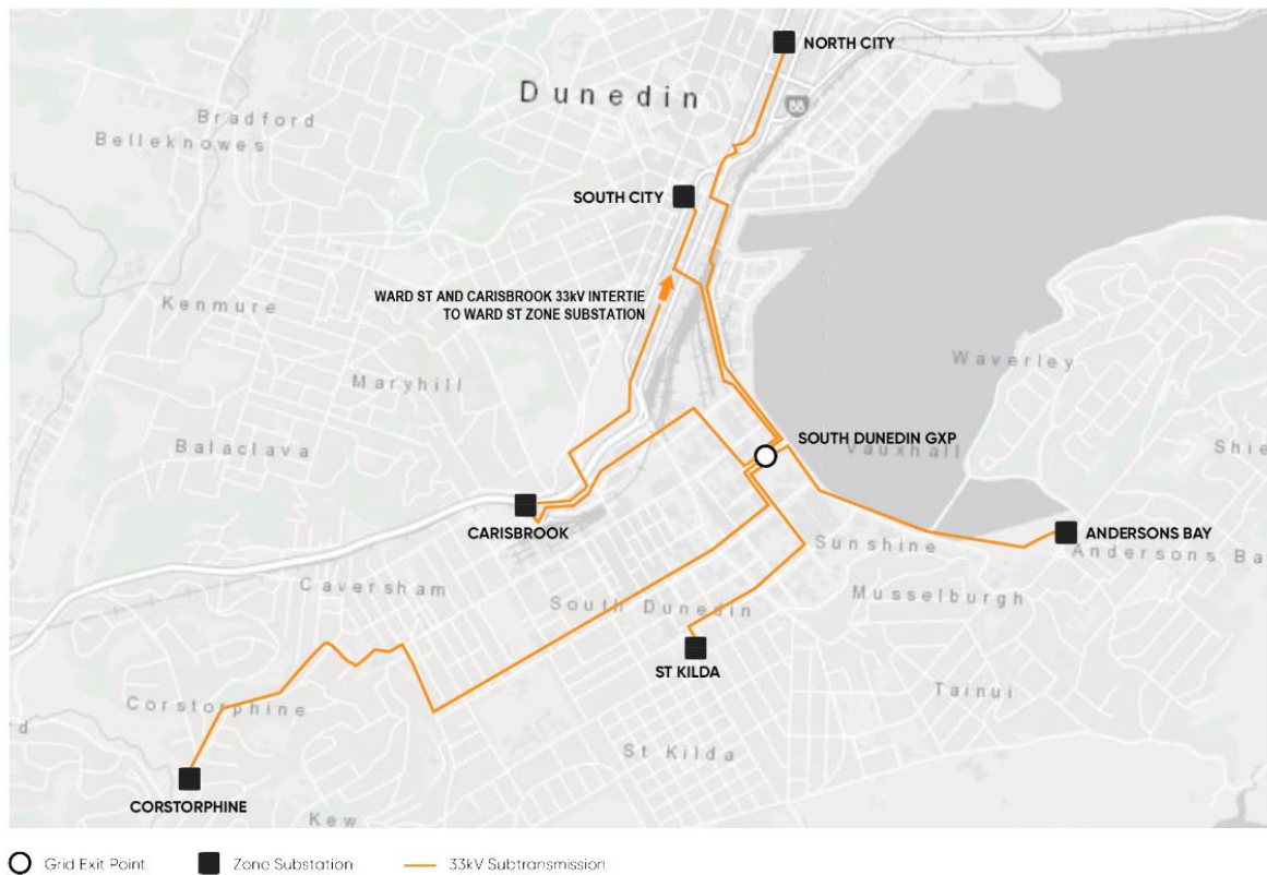
Figure 3.7: South Dunedin subtransmission network
