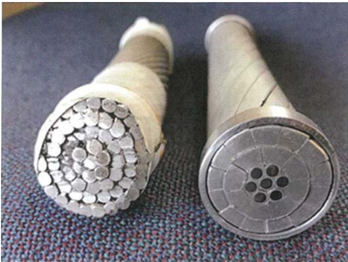
Stranded ACSR Zebra conductor (left) and trapezoidal ACSR Curlew conductor (right)
