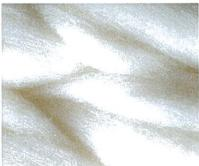
Following scouring which rids the wool of impurities, raw wool is carded and combed into tops: a large sliver of wool which is sold to spinners. Tops are made from blends, which ensure consistent production quality. Fibers are measured in microns which determine the final uses.
