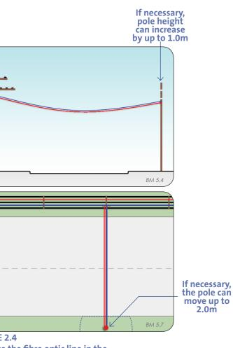
Route the fibre optic line in the telecommunications envelope only where an existing copper crossing occurs.
