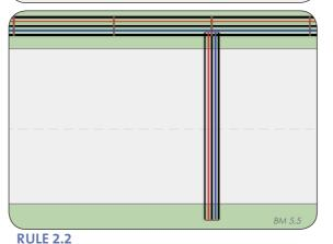
Route the fibre optic line under an existing electricity road crossing, within the telecommunications envelope.
