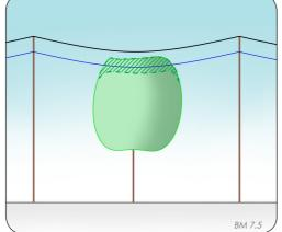
In situations where trees have already been pruned and/or require additional pruning, the works arborist will assess to determine whether the works fall within Class 1 or Class 2. In this example, works would result in more than 10% of the live canopy, and therefore would be assessed as Class 2.
