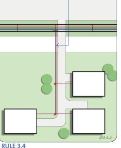
Fibre lines will follow existing copper lines along a ROW. Where possible, multiple lines will be combined into a multicore line.
