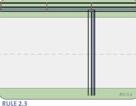
Route the fibre optic line in the low voltage electricity envelope.
