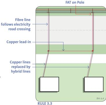
The final section of copper from the pole to the customer will be replaced by a hybrid line.
