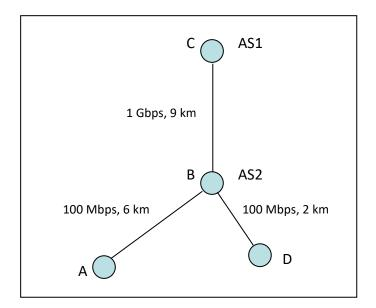
Note: The radial distances from A - B, B - C and D - B must be calculated separately to determine the applicable distance group for each Link.
