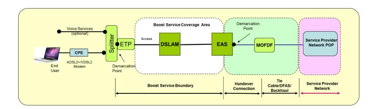
The following diagram provides a simplified overview of the physical components of the Boost Service when used with the Commercial Tail Extension Service.
