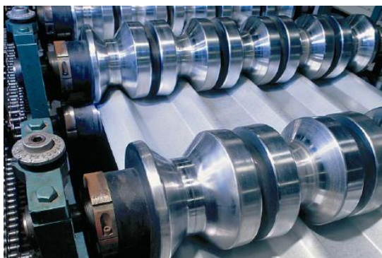
Roll forming ZINCALUME® steel for roofing
