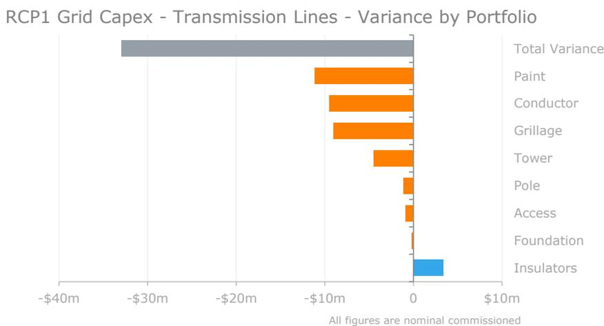
**Table 4: Transmission Lines (R & R) Capex during RCP1**
