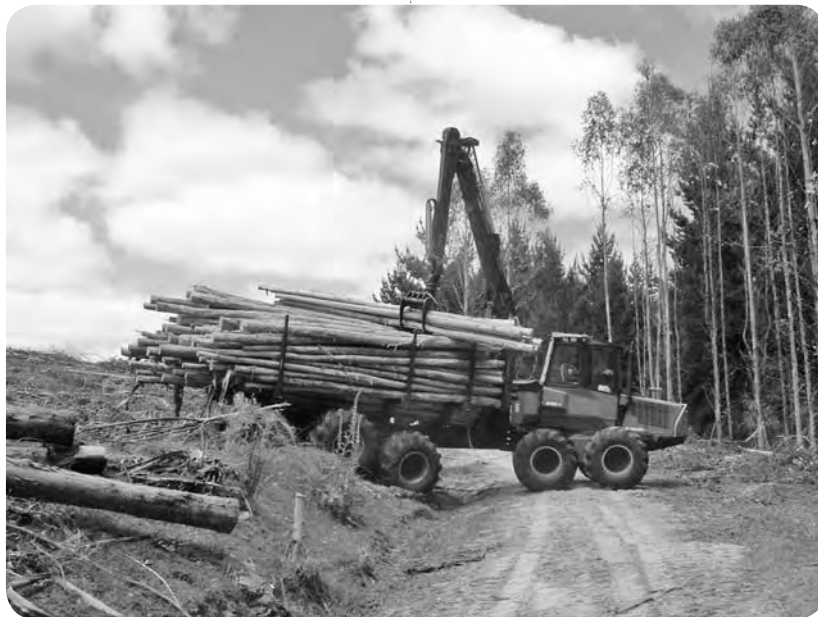
Forwarder loading eucalypt pulpwood at Wairakei Forest. Photo: David Little/Crown Forestry.
