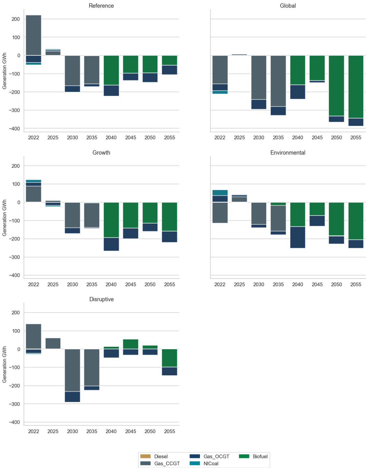
Figure 23: Yearly average fossil fuels and biofuels generation, counter factual vs preferred option factual (Tiwai leaves 2024 and HVDC fourth cable 2027)
