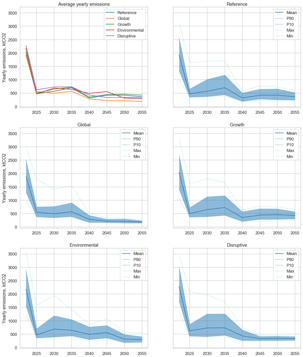
Figure 29: Yearly greenhouse gas emissions, preferred option with Tiwai leaves in 2024 and HVDC fourth cable in 2027
