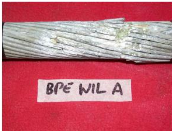
Figure 5- Example of dog done spacer damage as seen on the BPE-WIL A line
