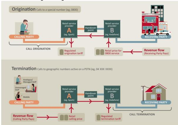
Figure 1: Origination and termination on a fixed PSTN
