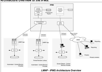
The architecture is based around a logically centralised IPMS node. Physically this may be mirrored to achieve the required Service Levels.
