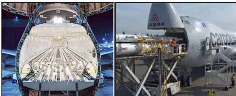
Left: Front image of a Boeing 747-8F, showing the freight capacity in its hold.
