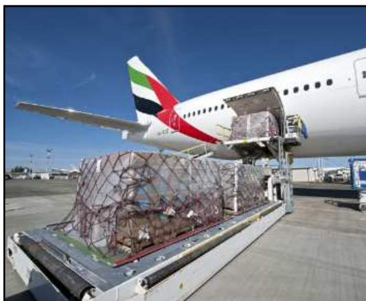
Above: Palletised cargo being loaded into the bellyspace of a Boeing 777-300 passenger jet.
