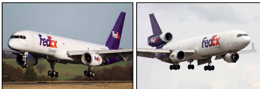
Two of FedEx's most commonly-used aircraft: Left: a medium range Boeing 757-200F; and Right: a wide-body McDonnell Douglas MD-11.
