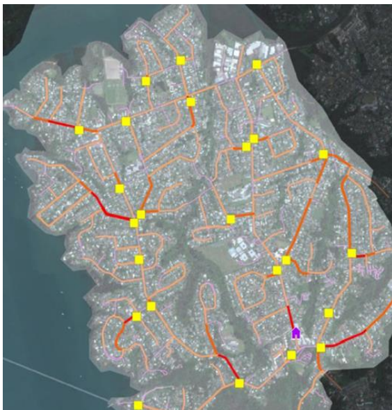
Figure 2.9: Illustration of concentration of cables in the modelled copper distribution network [Source: Model presentation, 2015]
