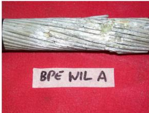
Figure 3 - Example of dog done spacer damage as seen on the BPE-WIL A line
