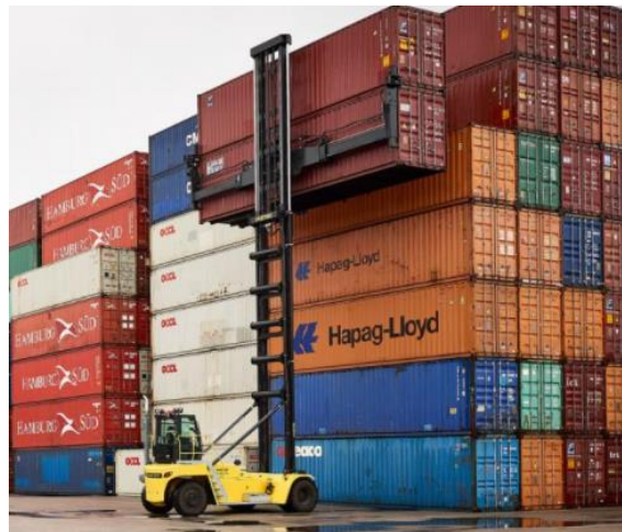
Figure 4: Empty container handler stacking two empty containers at a time
