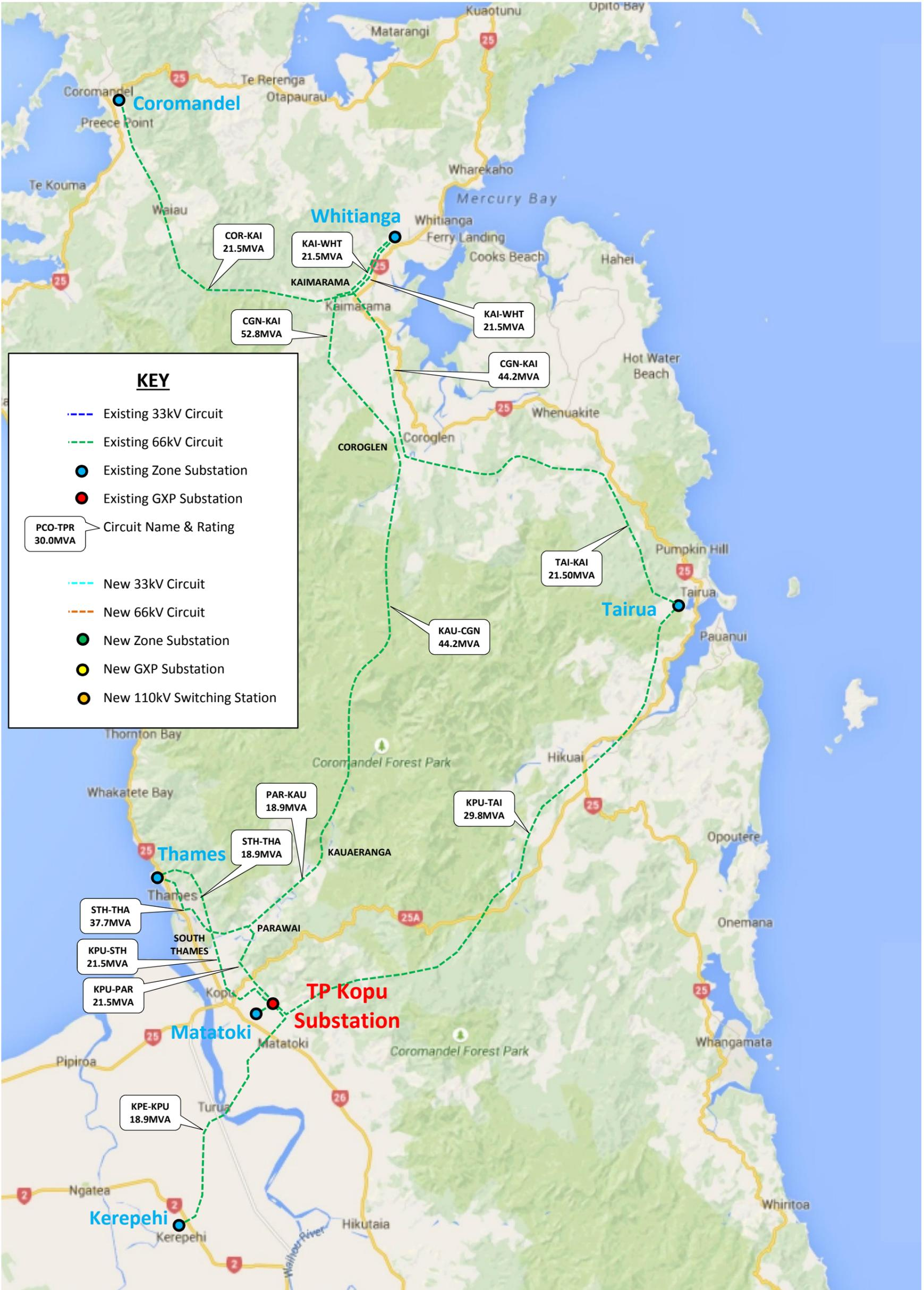
Figure 1: Existing Kopu GXP Sub-transmission Network: Geographic Diagram
