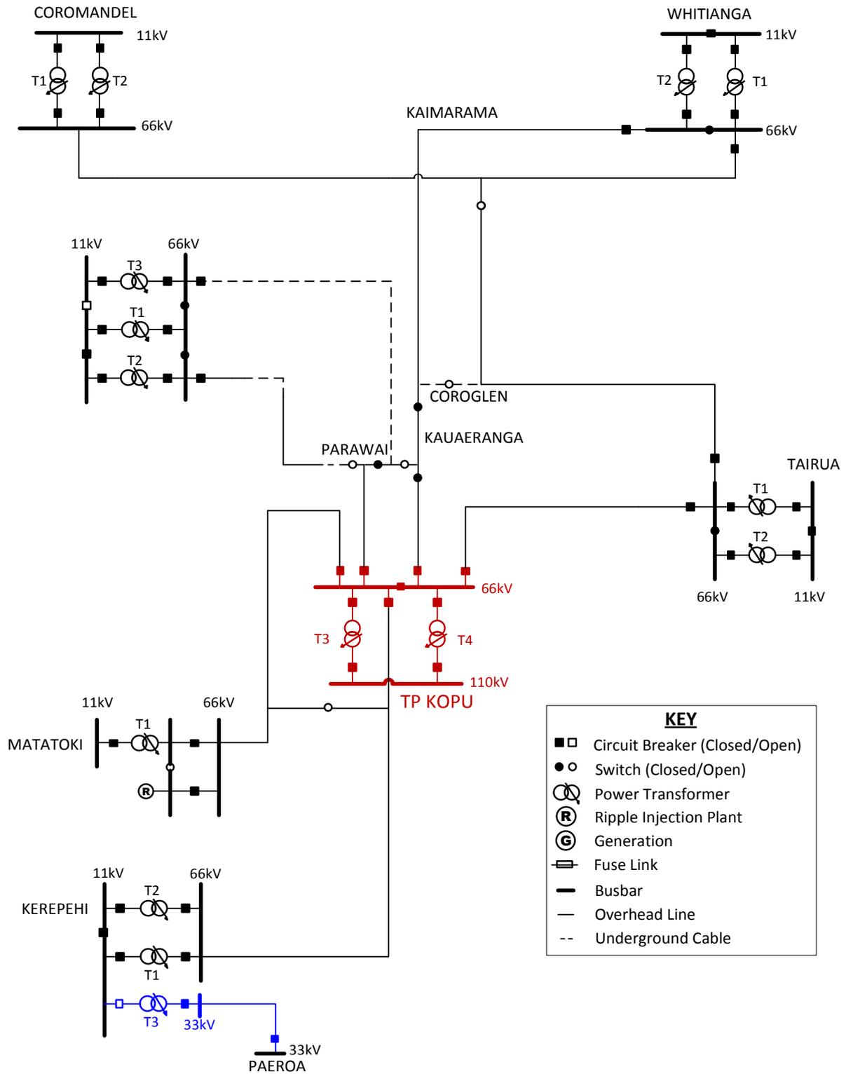
Figure 4: Option 6: Reinstate 50kV line to 33kV from Paeroa to Kerepehi substation: Single Line Diagram
