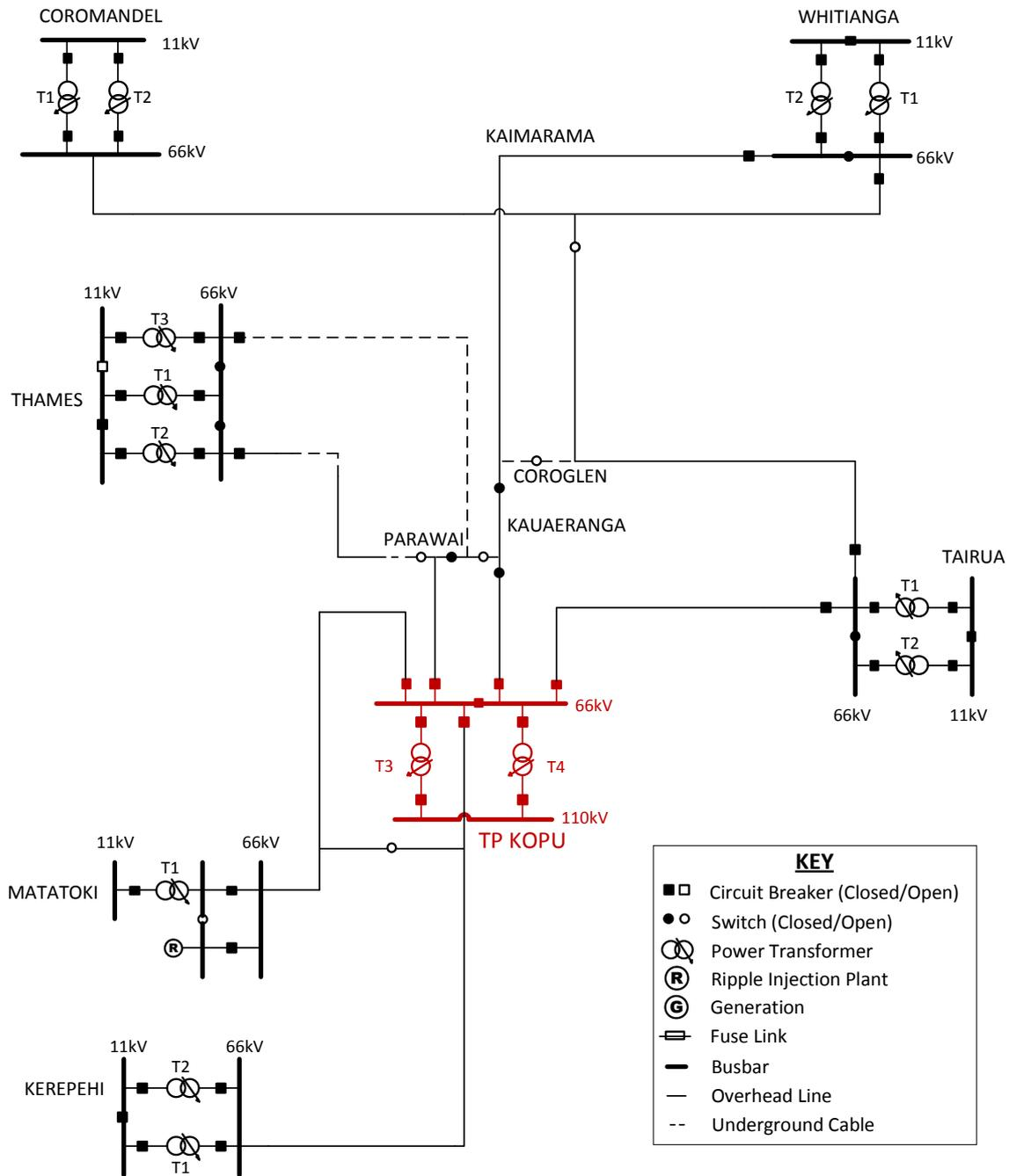
Figure 3: Existing Kopu GXP Sub-transmission Network: Single Line Diagram
