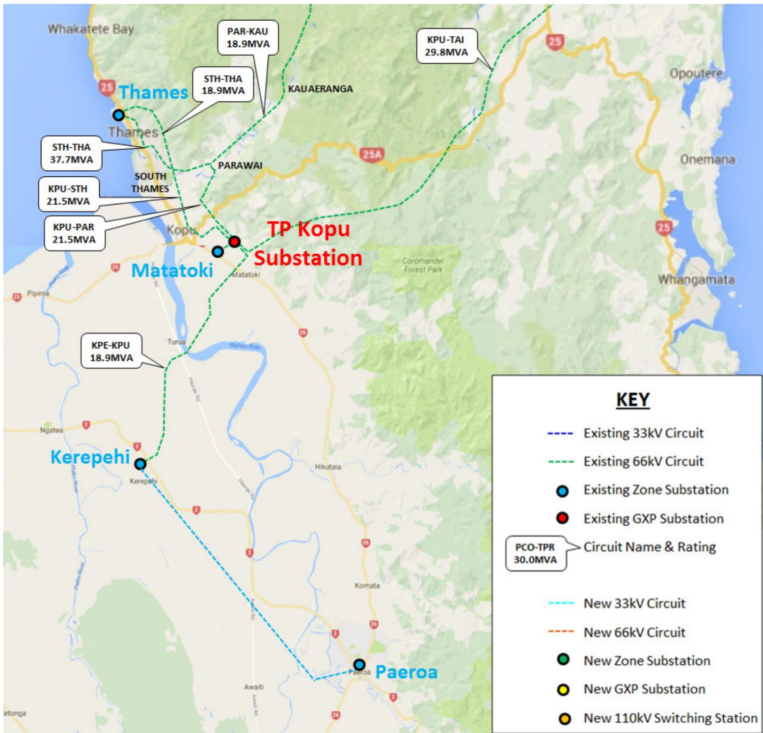
Figure 2: Option 6: Reinstating 50kV line to 33kV from Paeroa to Kerepehi substation Geographic Diagram
