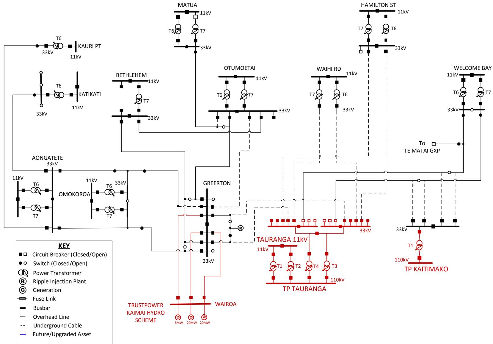
Figure 4 Existing Tauranga & Kaitimako Complete Sub-transmission Network: One-Line Diagram
