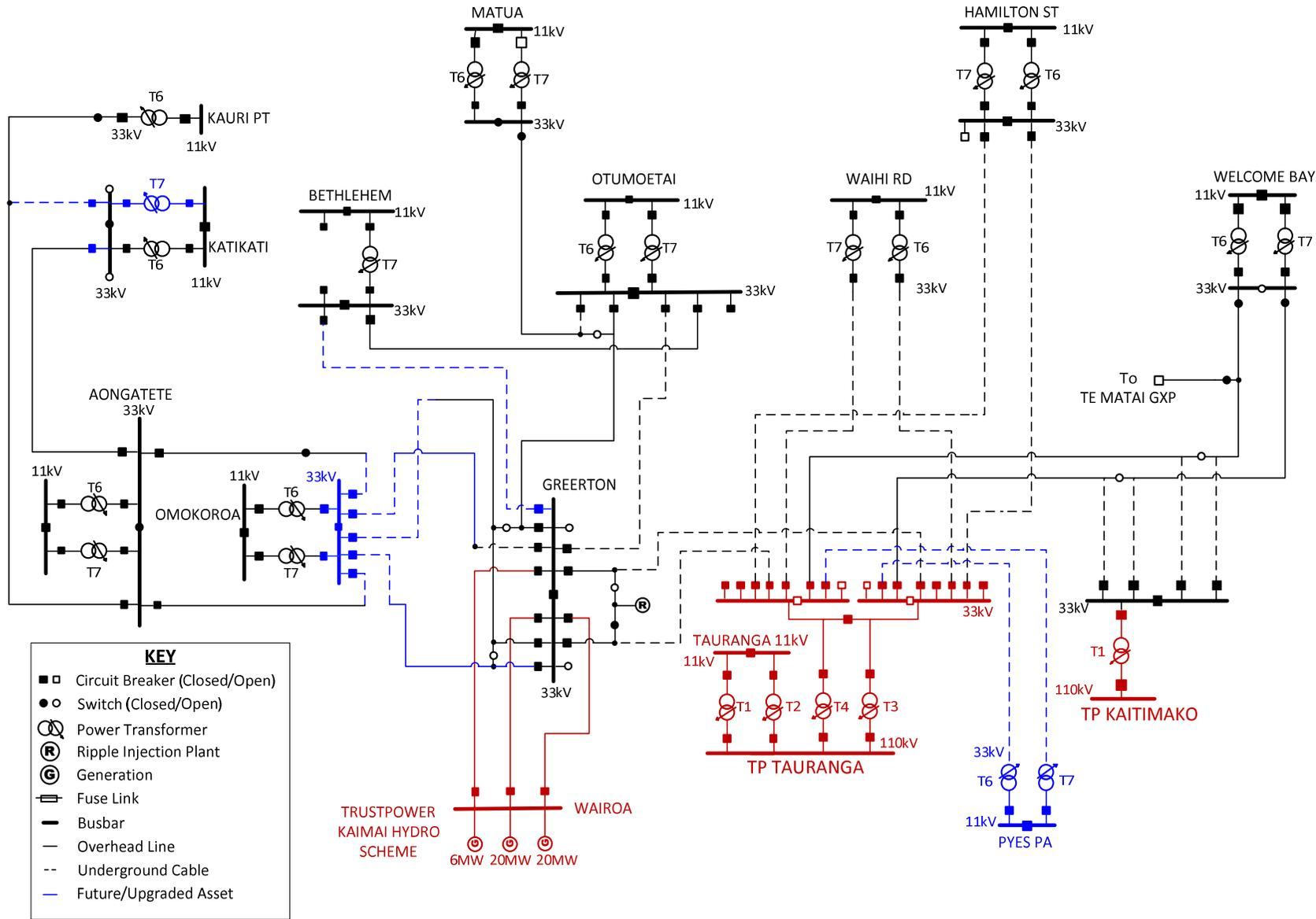
Figure 5: Option 5 – New 33/11kV Zone Substation at Pyes Pa- One-Line Diagram circa 2023
