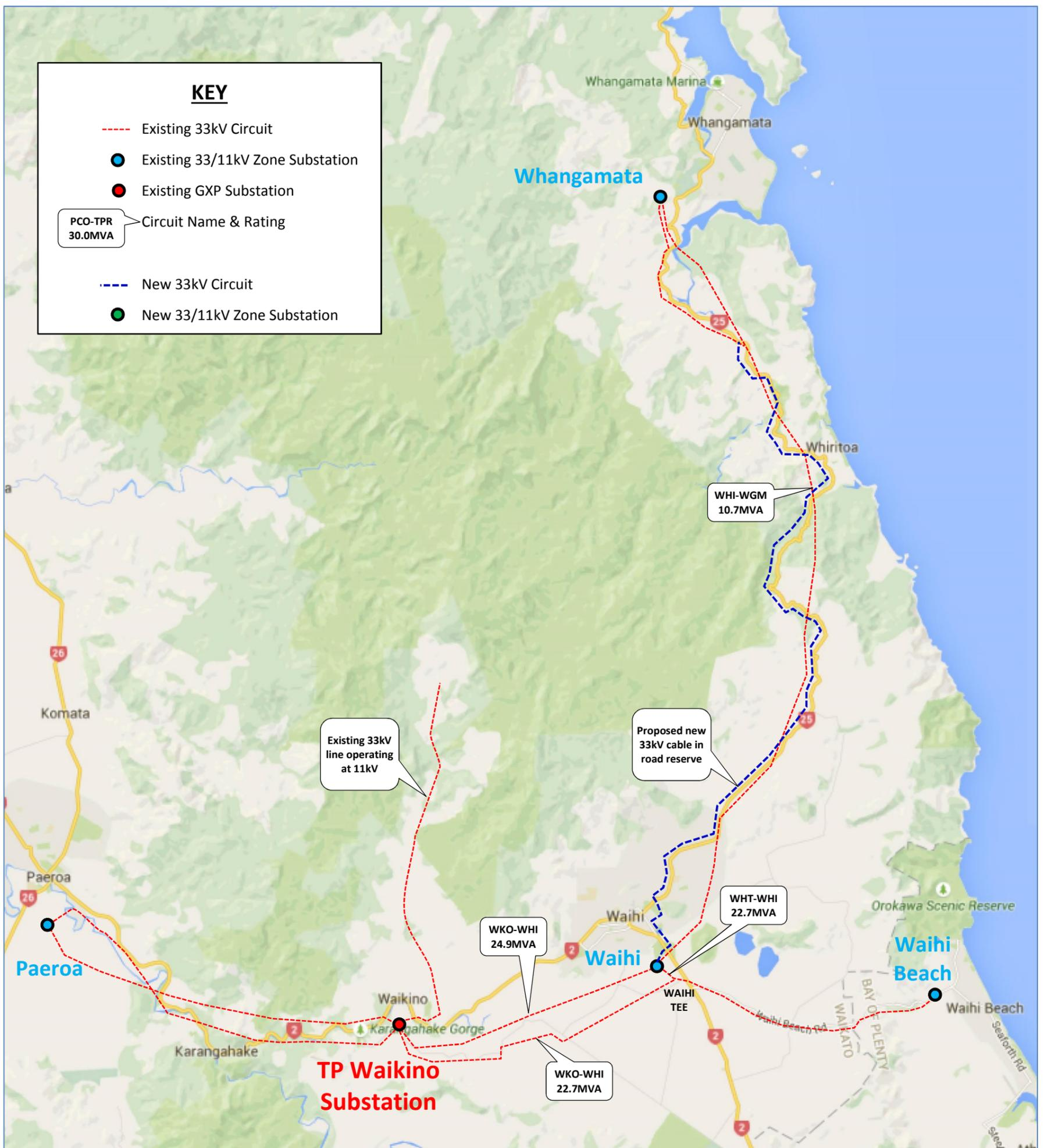
Figure 3 Option 5: New 33kV underground cable – Waihi to Whangamata: Geographic Diagram
