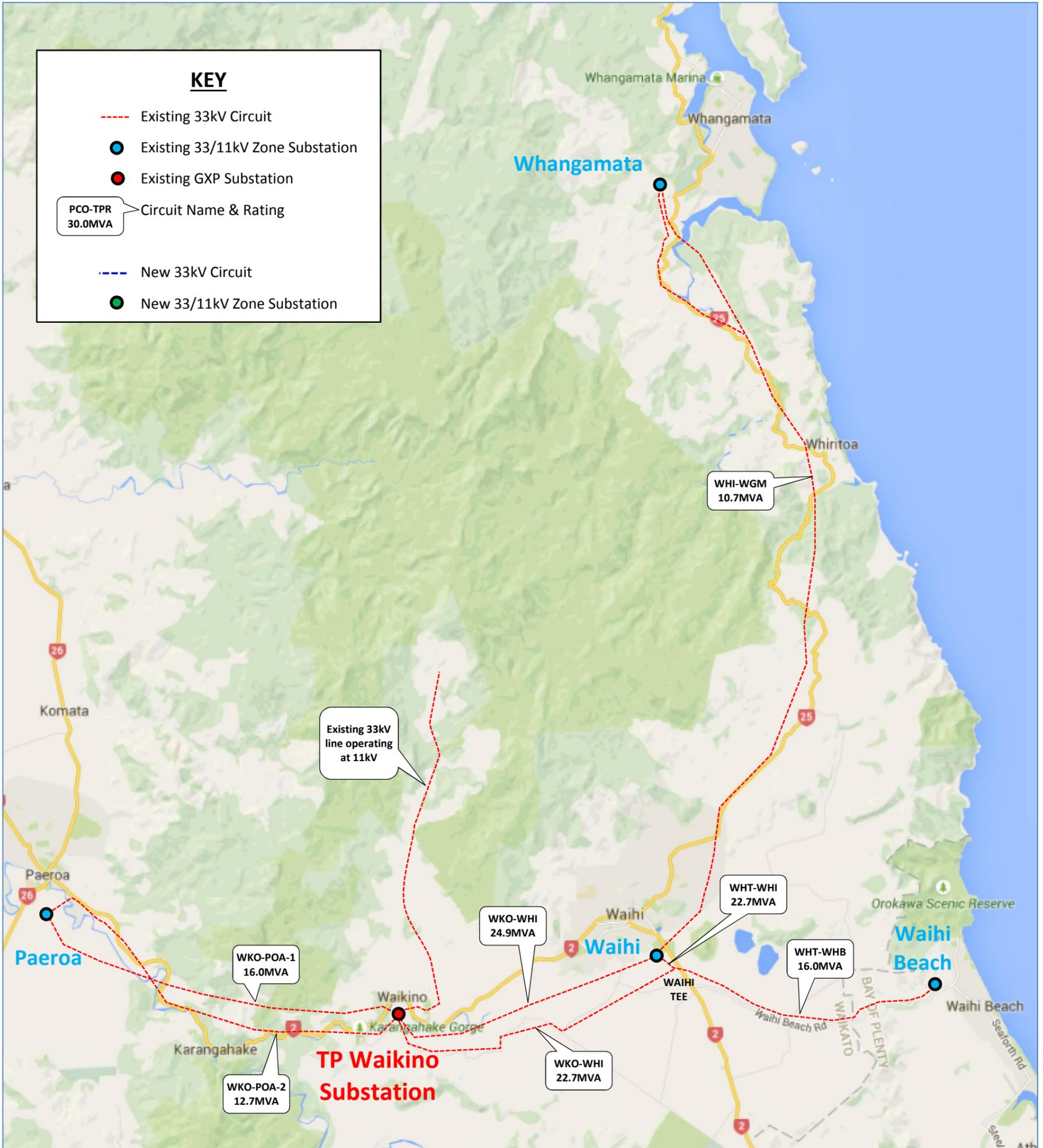
Figure 1 Existing Waikino/Whangamata Sub-transmission Network: Geographic Diagram
