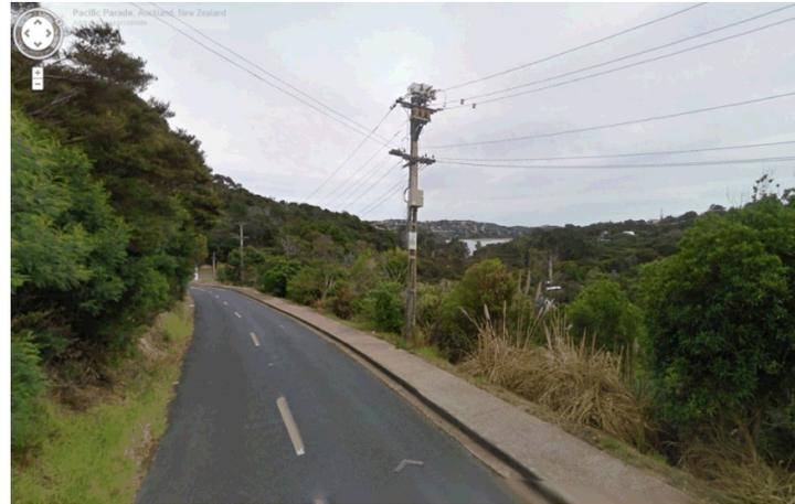
This example photograph shows a pole holding a Yagi antenna. The electricity lines company did not permit Chorus to utilise the pole, meaning the area needed to be undergrounded.
