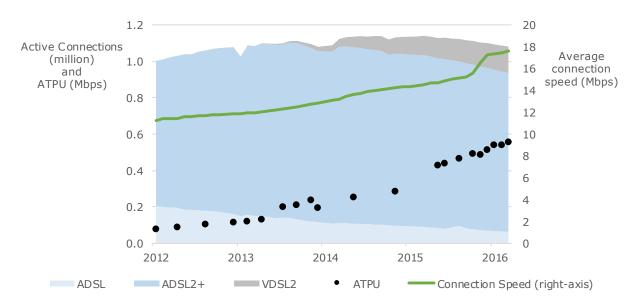
Figure 1: Broadband connection speeds and throughput (copper network)
