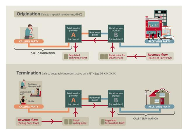
Figure B1 Origination and termination on a fixed PSTN
